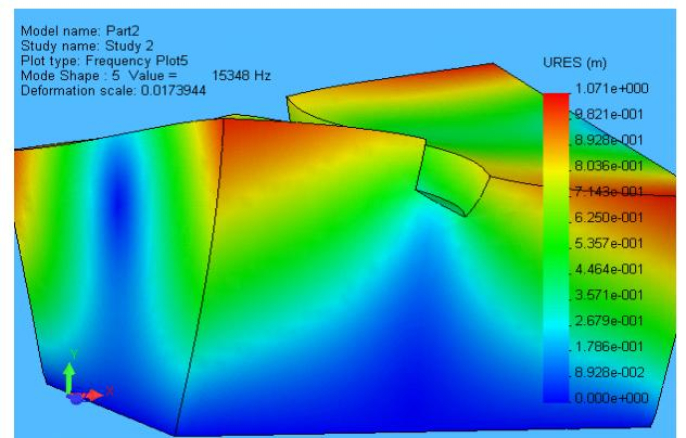
Figure 2. Interaction of a transverse grove with Rayleigh wave.
