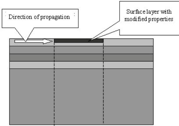
Figure 3. Longitudinal wave barrier.
