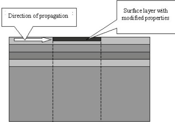
Figure 3. Longitudinal wave barrier.
