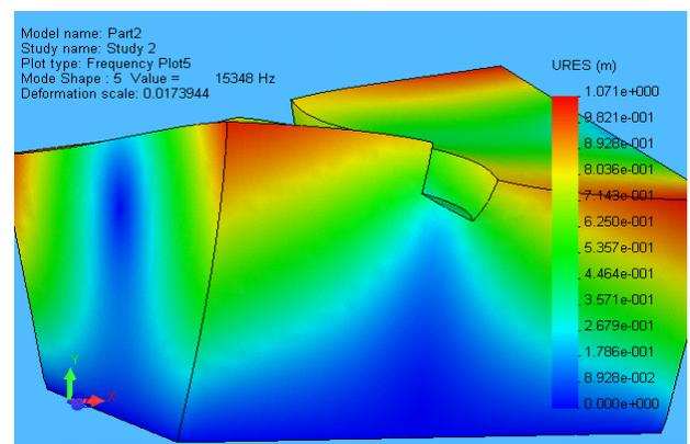
Figure 2. Interaction of a transverse groove with Rayleigh wave.
