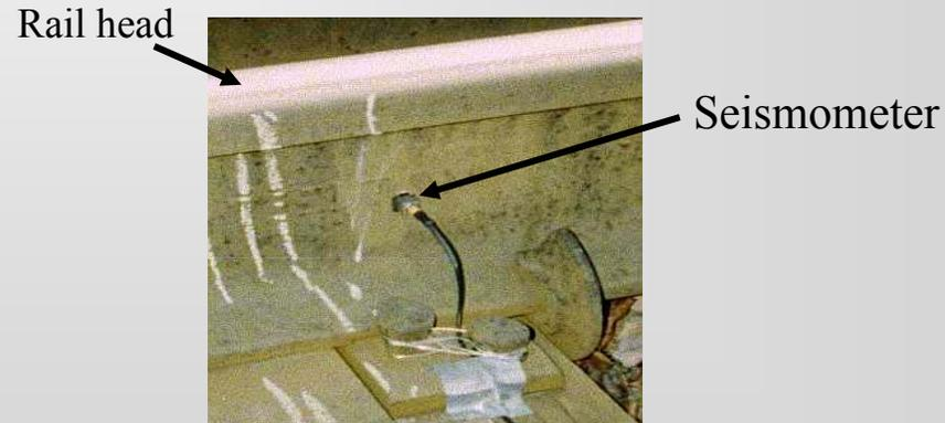
Crack determination in rails
