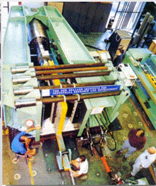
Two bearings, each weighing three-quarters of a tonne, are put through a seismic-simulation test rig
