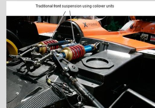
An example of horizontal displacement of dampers by “Racing for Holland” Co.
