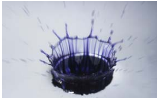
Discrete distribution of matter of impact droplet in the target fluid
